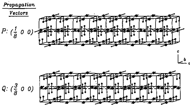
Figure 3. 3D model of the magnetic moment distribution of the two Fourier components of AFI. The moments of the component (\frac{1}{8}, 0, 0) are drawn too long (by a factor three) in comparison with those of (\frac{3}{8}, 0, 0) . The true magnetic structure is obtained as the vector sum of the Q component and \frac{1}{3} of the P component.
